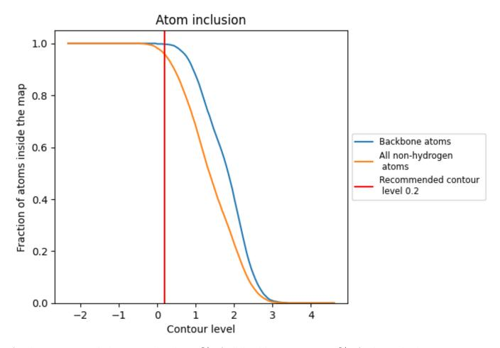
At the recommended contour level, 100% of all backbone atoms, 96% of all non-hydrogen atoms, are inside the map.
