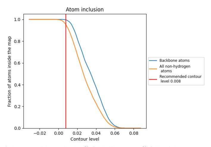
At the recommended contour level, 100% of all backbone atoms, 95% of all non-hydrogen atoms, are inside the map.
