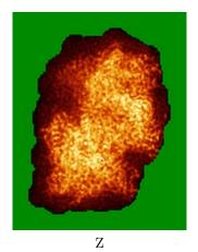
The images above show the map standard deviation projections with false color in three orthogonal directions. Minimum values are shown in green, max in blue, and dark to light orange shades represent small to large values respectively.
