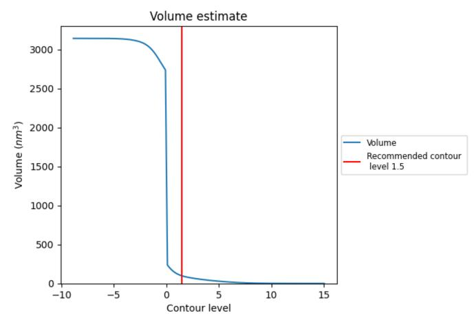
The volume at the recommended contour level is 98 nm<sup>3</sup>; this corresponds to an approximate mass of 89 kDa.
