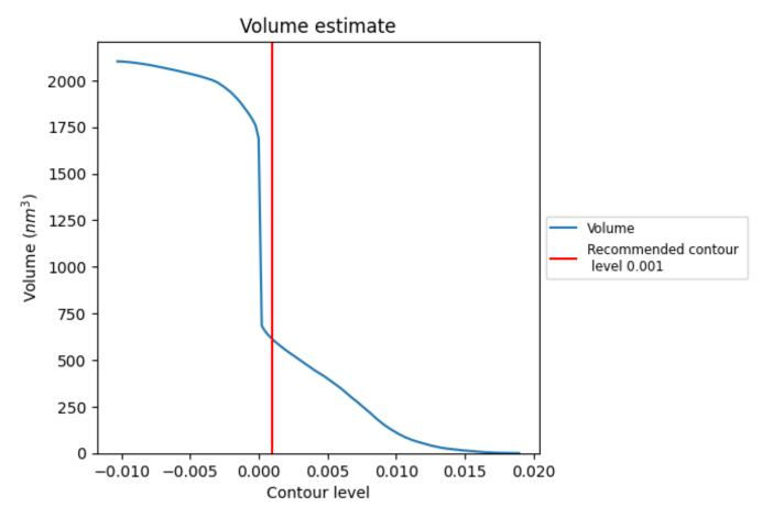
The volume at the recommended contour level is 611 nm<sup>3</sup>; this corresponds to an approximate mass of 552 kDa.
