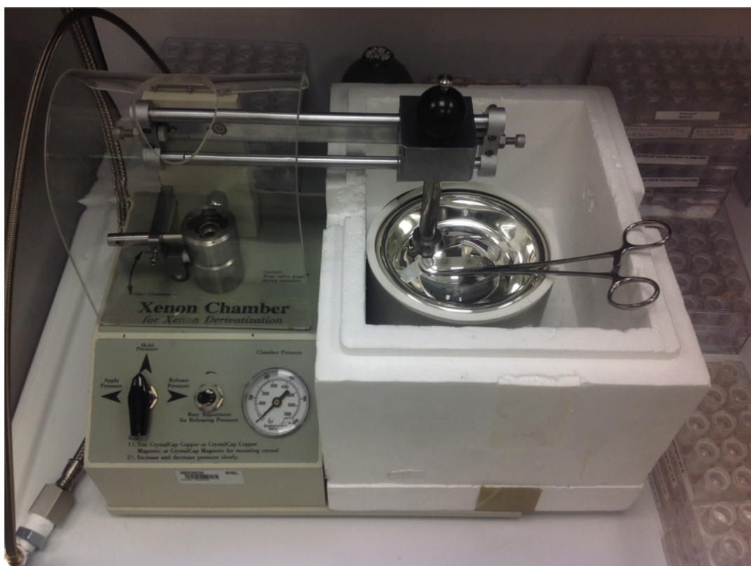
Figure 4.18 – Xenon pressure chamber used to expose protein crystals to xenon gas. Technical details and a schematic representation of the device can be found in Methods section 4.4.3 and Figure 4.29. Photo courtesy of Dr. Michele Cianci, EMBL Hamburg (Germany).
