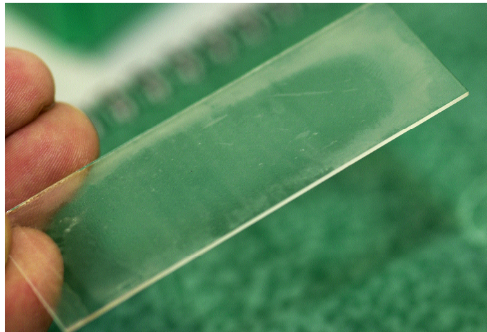
DNA chips are made by mounting molecular probes on ordinary glass slides.
